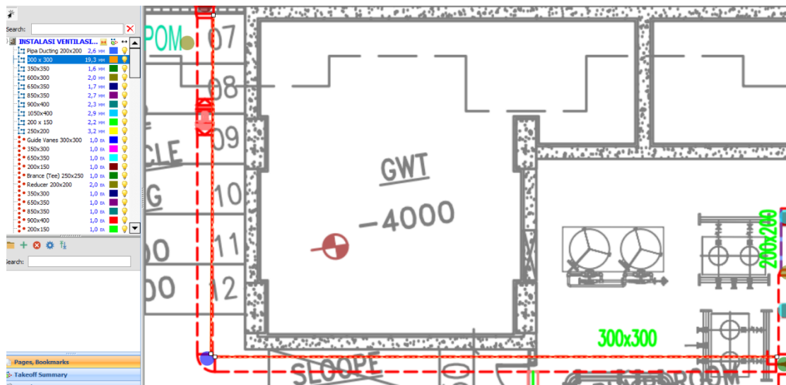
Gambar 3. 15 Gambar Denah AC Lantai Basement
