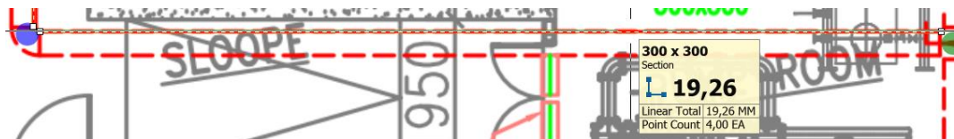
Gambar 3. 14 Contoh Ducting Ventilasi Lantai Basement
